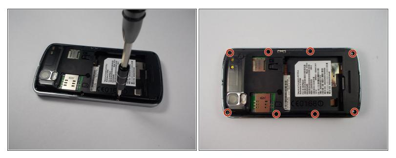
• Using a T4 Torx driver, remove the eight 4 mm back panel screws.
