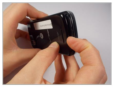
Remove the back cover using the thumb tab located on the bottom of the phone.
