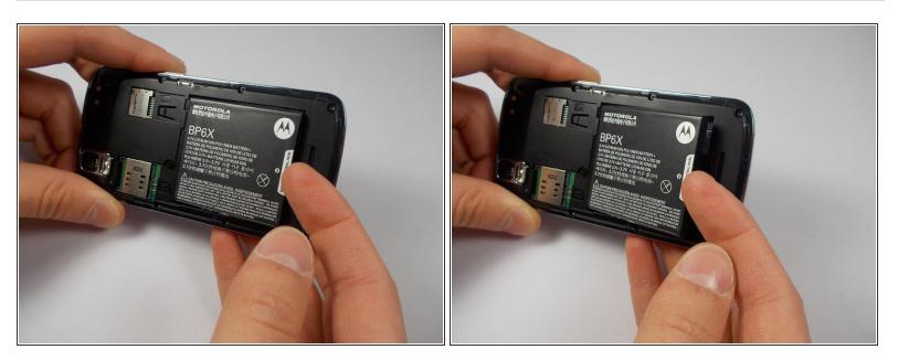
• Remove the battery using the thumb tab.
