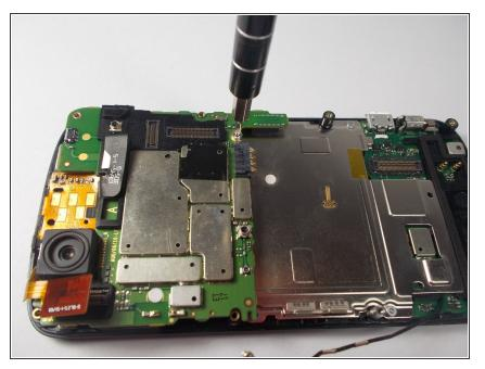
• Use a T5 Torx Screwdriver to unscrew the 2mm screw.
