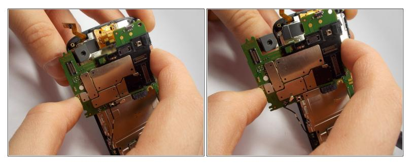
• To remove the motherboard, pull it to the side. The camera that is connected to the motherboard does not pull straight up and out from its holder.
