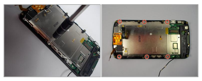
• Use a T4 Torx Screwdriver to remove the (6) 1mm screws.
