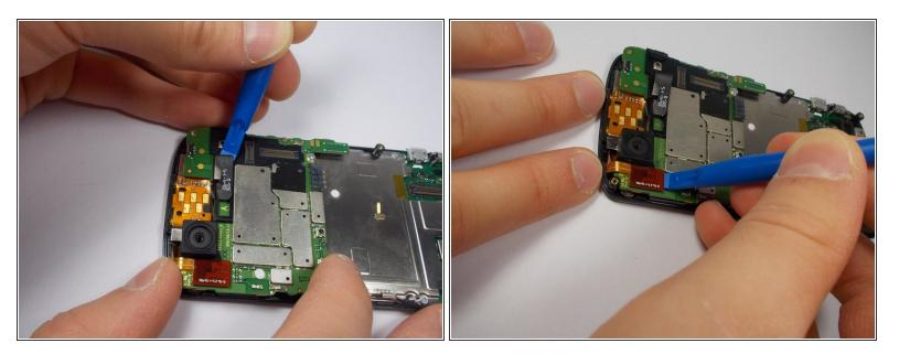
• Use your plastic opening tool to disconnect the two ribbon cables at the top of the phone.
