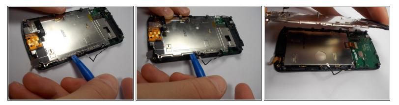
• Using a plastic opening tool or spudger lift the rear screen plate up and pull it off.
