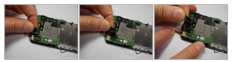
• Remove the camera's rubber seal by pulling it off. It is not connected to anything.
