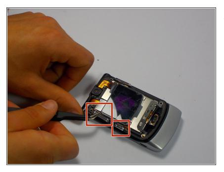
• Remove the two side buttons with tweezers.
