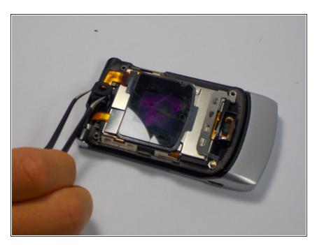
• Use tweezers to remove the circular magnetic ring covering the camera.
