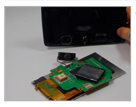
Replace the back cover screen, now that all parts have been properly removed.
