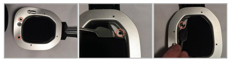
• Once the black plastic cover is removed, proceed to remove the two marked visible screws. Next peel back the foam in the top left and right corners of the speaker (the foam is glued on so be careful when removing it). During reassembly this will need to be re glued. once the screws are exposed remove them with the same screw driver.
