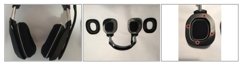
In order to replace the battery you must completely dissemble the ear piece with the mic. First remove the foam cushions from the ear piece. Do this by simply pulling the foam away from the ear piece. This will expose the 4 screws. Next Remove these 4 screws with a small Phillips head screwdriver.
