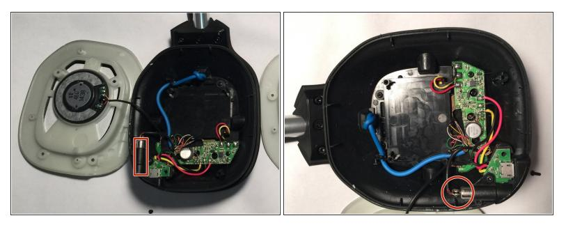
Locate the mic port and see if a wire is no longer connected to it. To reconnect the wire you will
