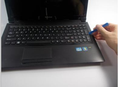
• Carefully pry off the keyboard with your plastic opening tool, moving along the edges.
