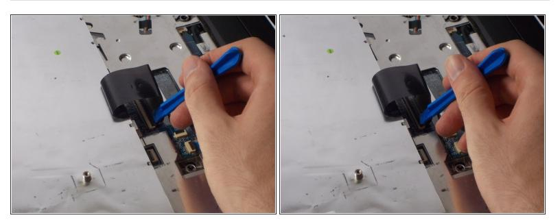
Use the plastic opening tool to lift open the ribbon connector that is holding the ribbon cable in its slot.
