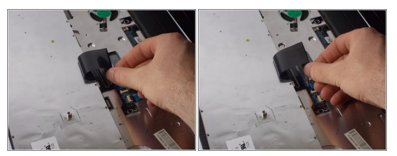
Remove the cable from its slot.
