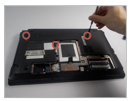
Remove the three 3 mm Phillips screws holding the keyboard in.
