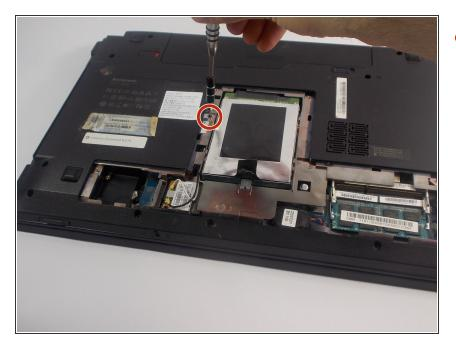
Unscrew the one 4 mm Phillips screw that is securing your DVD drive to the frame.
