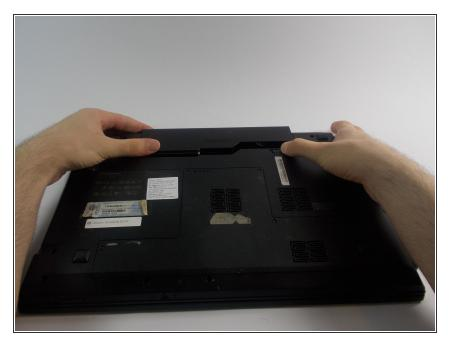
• Hold the right battery lock open with one hand while removing the battery itself with the other.
