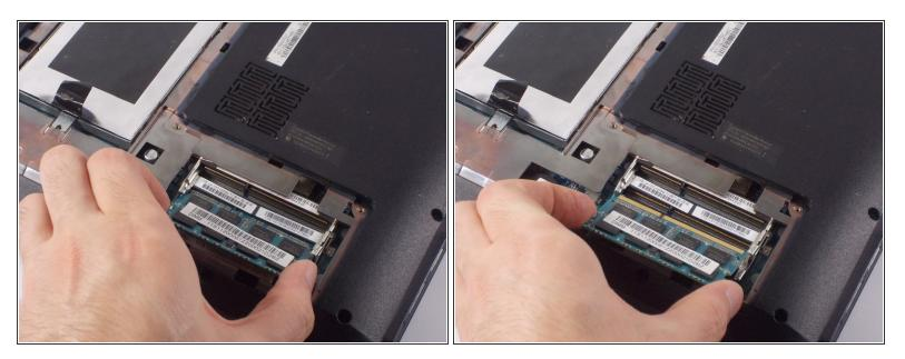
• Remove RAM by carefully pulling it away from its socket.
