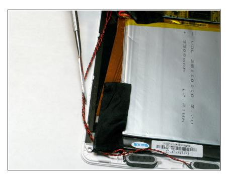
• Follow the speaker wires down to the speakers at the bottom of the tablet.
