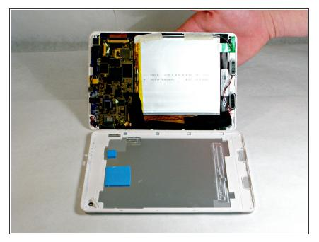
• You should now be able to separate the two halves of the tablet. Also place the back cover aside since you will no longer be needing it until reassembly.
