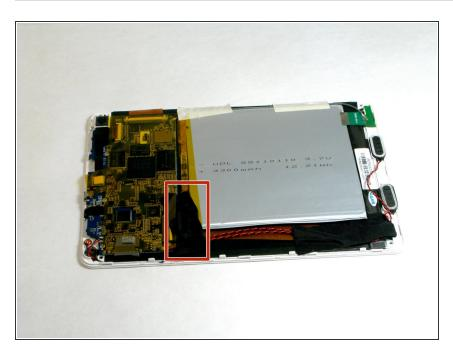
• With the motherboard facing upwards, locate the speakers and the Braided (Red and Black) wires connecting them. Once located remove the two pieces of black adhesive tape retaining the wires using a small pry tool or your hands.
