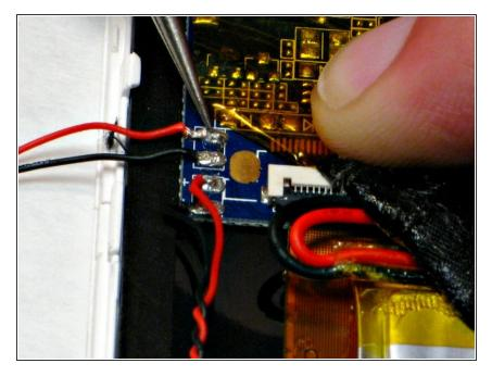
Re-soldering is the same process as de-soldering, except you will also add solder. Be sure to be precise and clean when soldering. Look up soldering tutorials for help on youtube if you do not feel comfortable. Once all wires are resoldered reassemble the tablet following the steps in reverse order.
