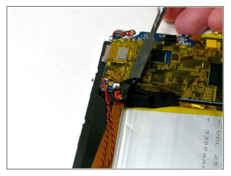
Once removed you will notice the solder locations that connect the Braided (Red and Black) wires to the motherboard.
