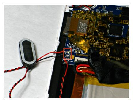
Look closely at the soldering points. Take note of how the positive(Red) and negative(Black) connections are placed on the motherboard. With your soldering iron carefully heat the solder point until it begins to melt.
