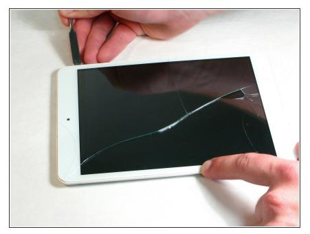
• Starting near the middle edge of the Trio Stealth-G4X tablet, gently work the small pry tool in between the seams of one side of the tablet.
