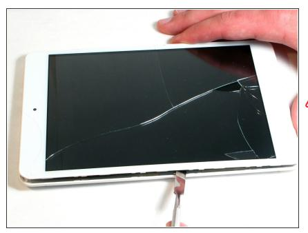
Work your way around all four corners of the tablet, unlocking all of the retaining tabs that hold the tablet together.
