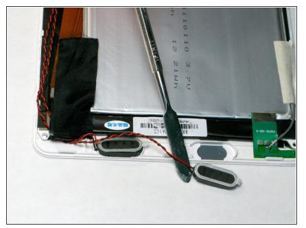
Use the pry tool to gently loosen the speakers out of place. Once loose separate the two sets of speakers so that you can identify which one must be replaced and which solder points you must <u>desolder</u> in the next steps.
