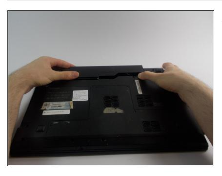
Hold the right battery lock open with one hand while removing the battery itself with the other.
