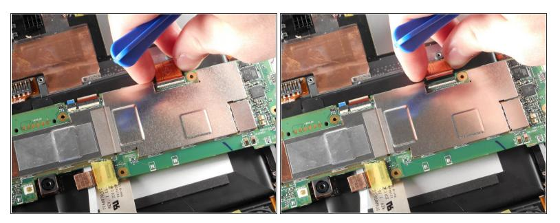
Gently remove the charging port ribbon piece from the motherboard. It should come out easily using your fingers.
