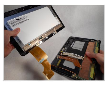
Lift the screen upwards to remove.
