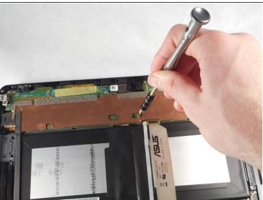
Remove the eleven 0.79 mm #000 screws around the motherboard with the Phillips #000 screwdriver.
