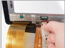
With all three white levers pushed in, gently pull on each display cable until the cable disconnects.
