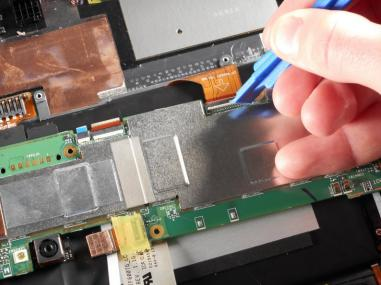
Flip up the white lever with the plastic opening tool to release the connection.
