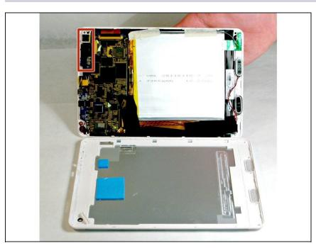
Once the two halves are separated, set aside the back cover of the tablet as you will not need it until reassembly. Now locate the camera on the motherboard of the tablet.
