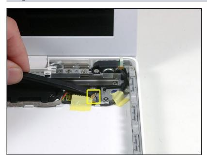
Use a spudger to disconnect the gold Bluetooth antenna connector from the Bluetooth board.
