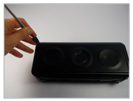
Push the nylon or metal spudger in the corner of the speaker guard.
