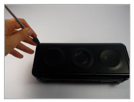
Push the nylon or metal spudger in the corner of the speaker guard.
