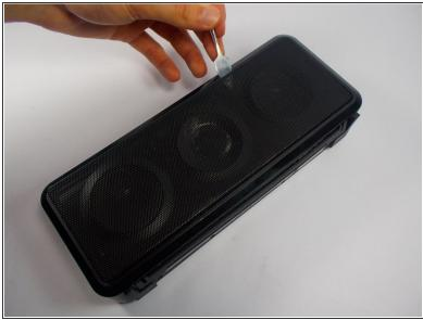
Slide the nylon or metal spudger all around the speaker guard.
