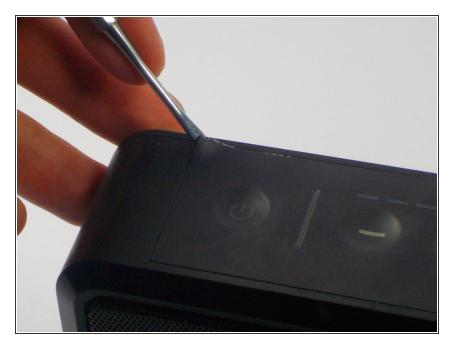
Push the nylon or metal spudger under the corner of the control pad.
