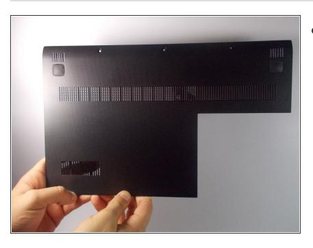
Slide, do not lift, the bottom panel off once the 3 screws are off.
