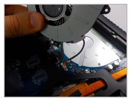
Once the screws are removed slowly lift the fan out, there will be a thin wire connected to the device and fan still, Firmly grasp the white end of the wire where the wire splits into 2 and pull it out.
