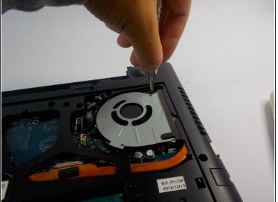
Remove the 3 screws attaching the fan to the device.
