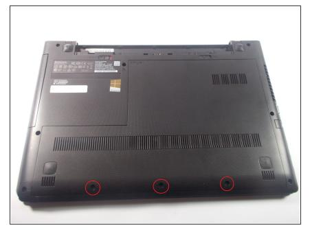
Safely flip the device upside down and use the Phillips head screwdriver to remove the 3 screws at the bottom of the device which are circled.
