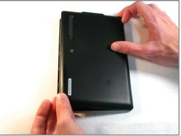
With your fingers, carefully pry off the back plastic casing. Starting at the corners is usually the easiest.
