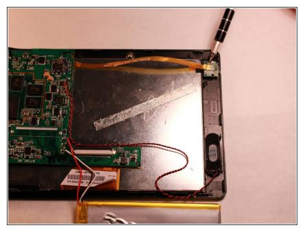
Remove the two screws that hold the audio jack in place. Carefully lift the audio jack out of the compartment.
