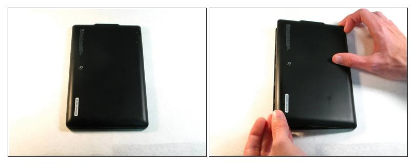
• With your fingers, carefully pry off the back plastic casing. Starting at the corners is usually the easiest.
