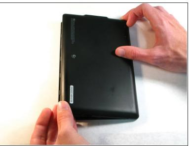
With your fingers, carefully pry off the back plastic casing. Starting at the corners is usually the easiest.
