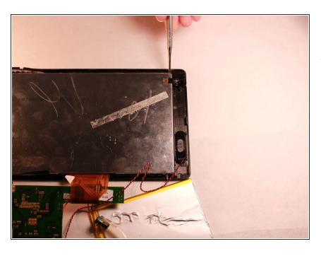
Use the Small Pointed Metal Spudger to separate the LED screen from the front screen by gently wedging the spudger between the screen and the device.
