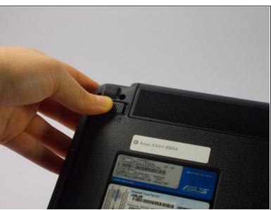
Slide the left lock button into the unlock position and hold.
