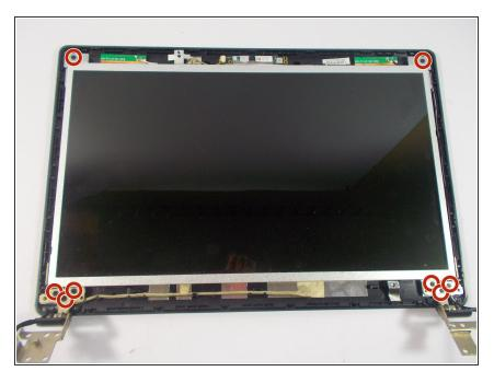
Remove the eight 5mm Phillips head screws holding down the screen with the PH0 bit.
