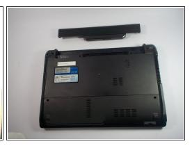
While holding the left lock button in the unlock position, push the battery from the center away from you.
