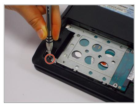
Remove the 9mm Phillips head screw in the left bottom corner of the hard drive with the PH0 bit.
