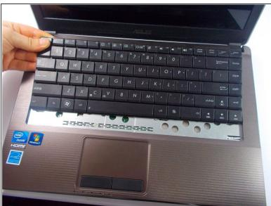
Push the keyboard away from the mouse track pad to unlock the bottom from the base.
