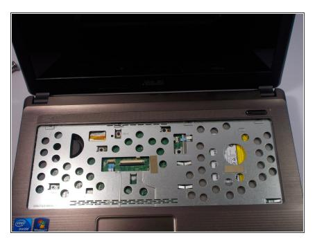
Remove the keyboard completely.
