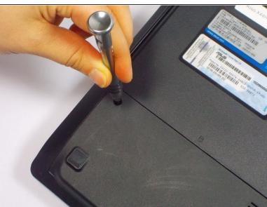
Remove the two 9 mm Phillips head screws with the PH0 bit indicated by the red circles in the picture.
