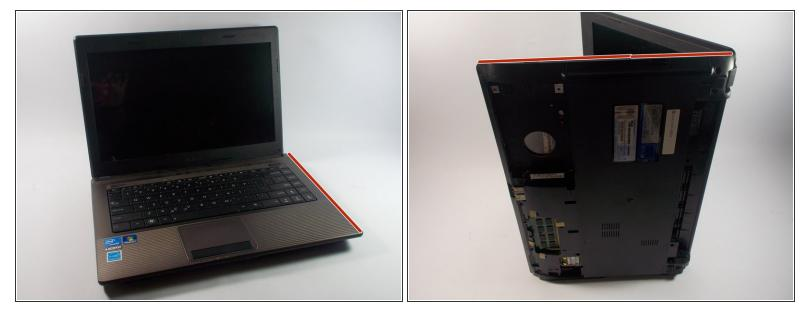
Flip the laptop on its side so that the red line indicated in the pictures is facing upwards.
