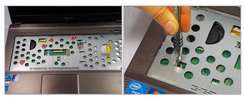
Remove the five 9 mm Phillips head screws with the PH0 bit.
