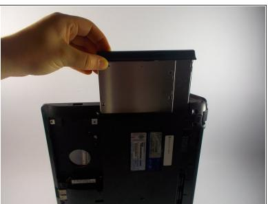
Pull up on the disk drive and remove.
