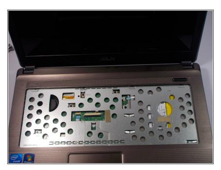
Remove the keyboard completely.
