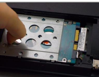
Slide the hard drive to the left, unlocking it from its default position.
