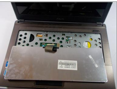
Flip the keyboard over to reveal the back of it and what is underneath.
