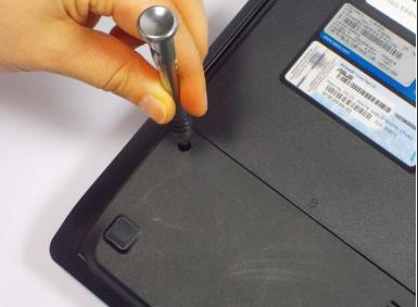
Remove the two 9 mm Phillips head screws with the PH0 bit indicated by the red circles in the picture.
