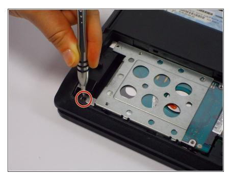
Remove the 9mm Phillips head screw in the left bottom corner of the hard drive with the PH0 bit.
