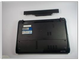
While holding the left lock button in the unlock position, push the battery from the center away from you.
