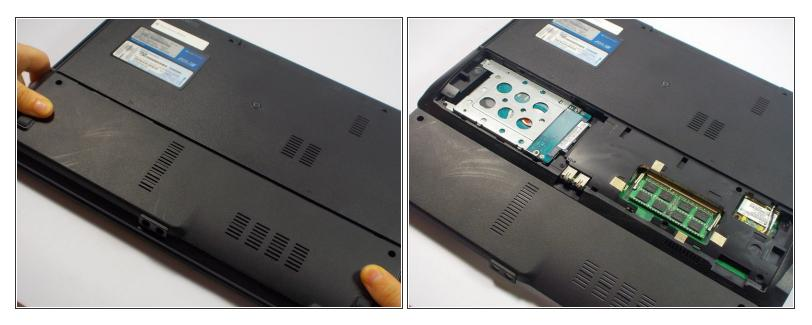
• Once the screws are removed, slide the back panel away from the computer.
