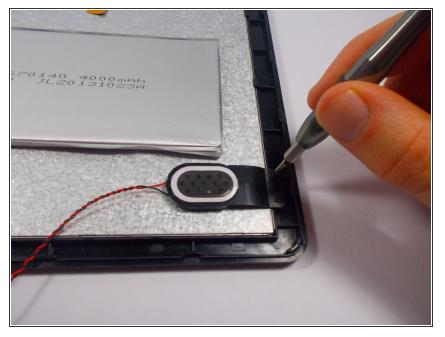
Next you will need to remove the two screws attached to the speaker. If you have a 54 bit Driver Kit use the Philips Head 0 (or PH 0) head to remove the two 4mm screws.
