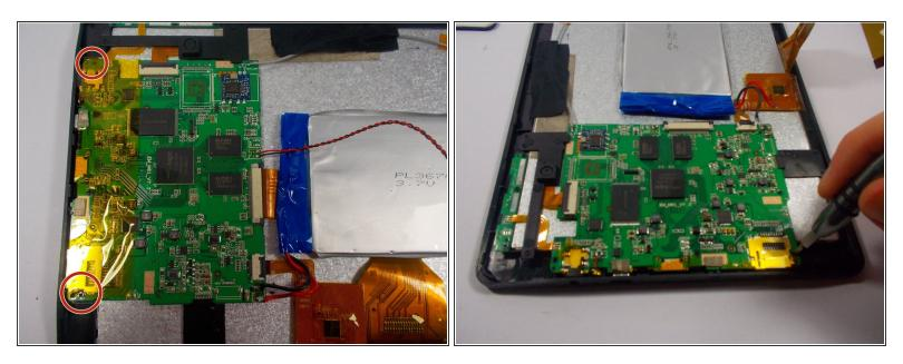
Use a Phillips #0 to unscrew the 4mm screws from the motherboard fixture.
