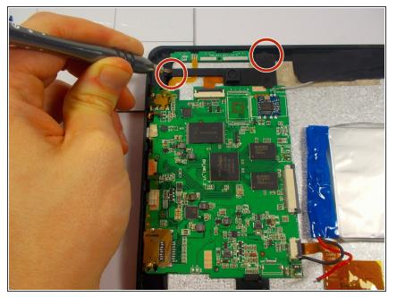
Next use your PH 0 to remove the two 4mm screws to detach the camera support fixture.
