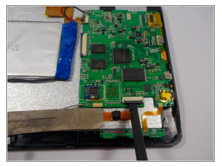
Disconnect the camera from the mother board. Use a spudger and lift the grey latch until it is facing up then pull out the connection for the cameras.
