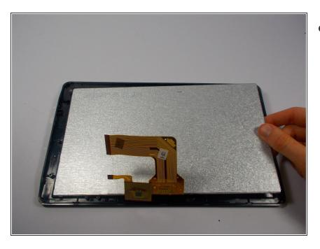
Remove all disconnected components and remove screen/digitizer.
