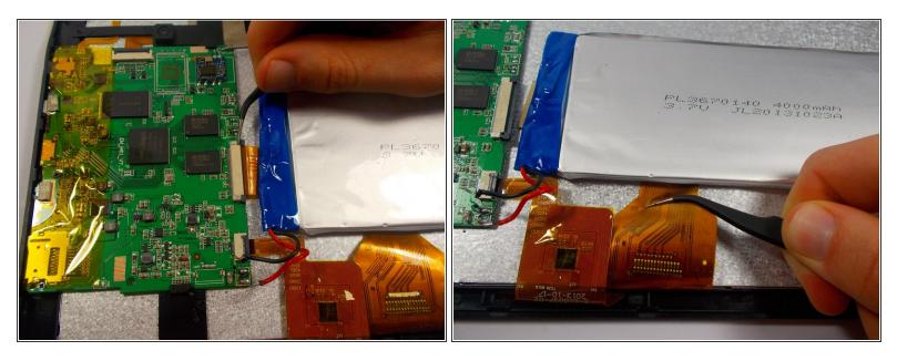
Use a pair of tweezers to grasp the screen/digitizer connection gently and remove each accordingly.
