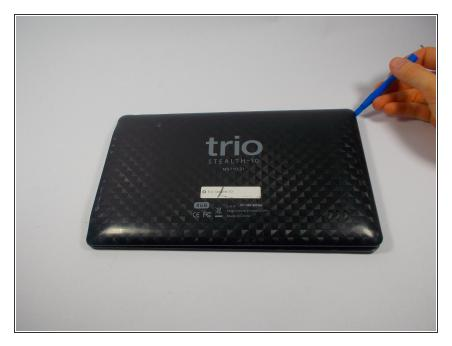
To remove the back panel, you will need to use a plastic opening tool and slowly separate the back panel from the device.
