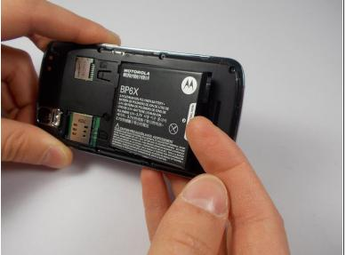
Remove the battery using the thumb tab.
