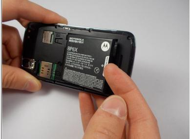
Remove the battery using the thumb tab.
