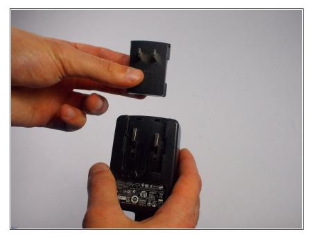
Remove the prongs from the AC Adapter. Any repairs on the prongs can now be easily done.
