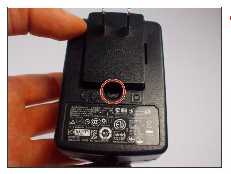
Locate the small hole, which is in the shape of a semicircle. It is below the plastic piece that has the prongs attached.
