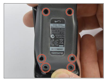
Using a size #000 Phillips screwdriver, remove the six 5 mm screws on the back of the device.
