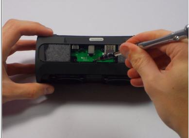
Remove the one screw holding the circuit board.
