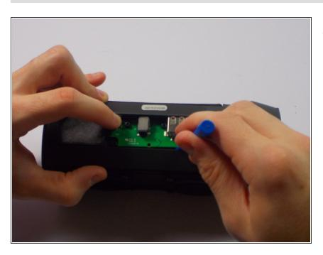
Pry the board with the plastic opening tool.
