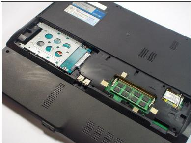
Once the screws are removed, slide the back panel away from the computer.
