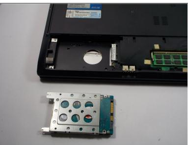
Pull the hard drive upwards and take it out of its position.
