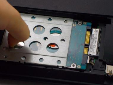
• Slide the hard drive to the left, unlocking it from its default position.
