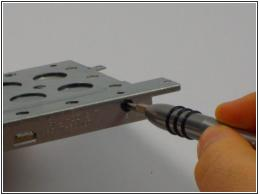
Remove two 3mm Phillips head screws, one located on each side of the metal casing holding the hard drive using the PH0 bit.
