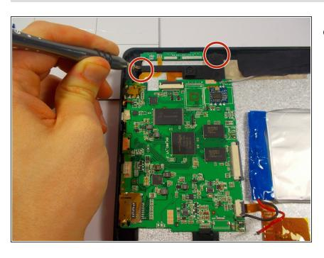
Next use your PH 0 to remove the two 4mm screws to detach the camera support fixture.
