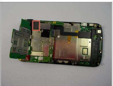
Gently lift the SD & SIM card board (PCB) as shown.
