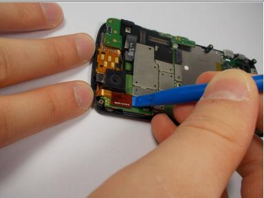
Use your plastic opening tool to disconnect the two ribbon cables at the top of the phone.
