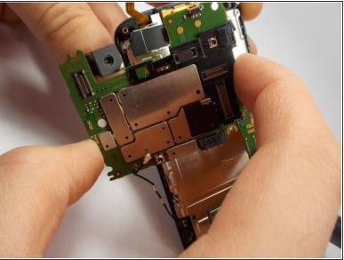
To remove the motherboard, pull it to the side. The camera that is connected to the motherboard does not pull straight up and out from its holder.
