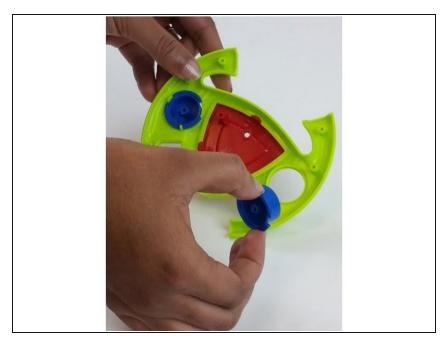
Open the remote control and remove the blue circular plastic buttons located on the right and left side on remote.
