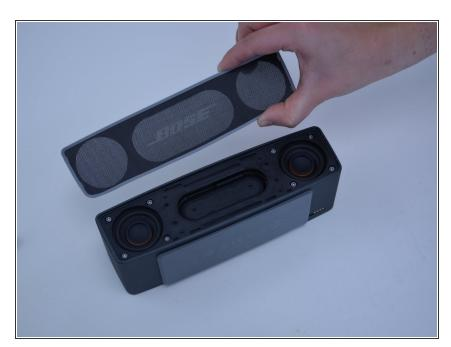
Remove the mesh tabs from the other side of the device.
