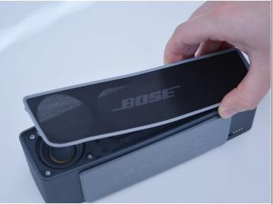
Carefully peel the mesh speaker guard away from the device.
