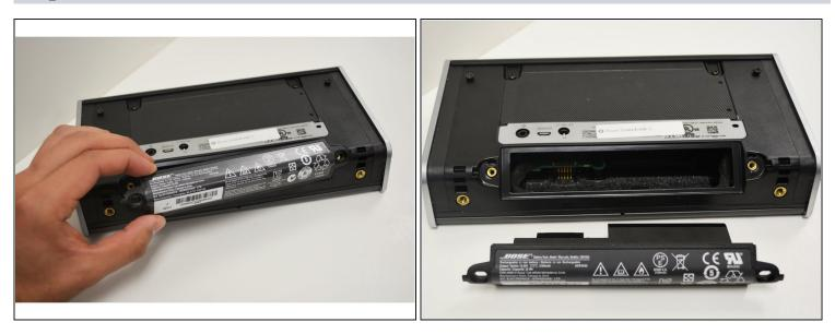
• Carefully remove the battery by pulling it out of the speaker.
