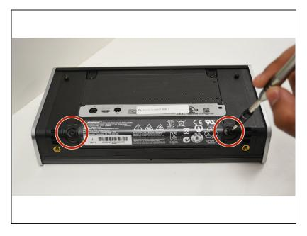
• Using the screwdriver with the T-10 star tip, remove the 6.75 mm. screws marked in red.
