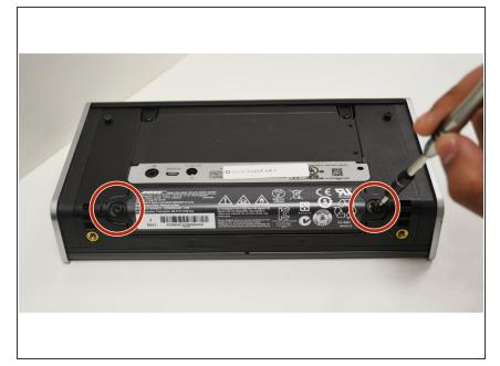
Using the screwdriver with the T-10 star tip, remove the 6.75 mm.
