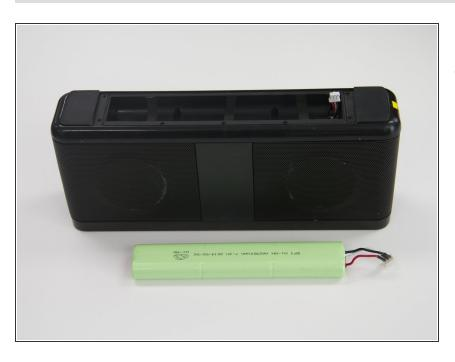
The battery is now separated from the device and may be replaced with a new battery. To reassemble your device, follow these instructions in reverse order.
