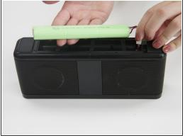
Starting from where the wires are connected, gently pull the battery out of the device.
