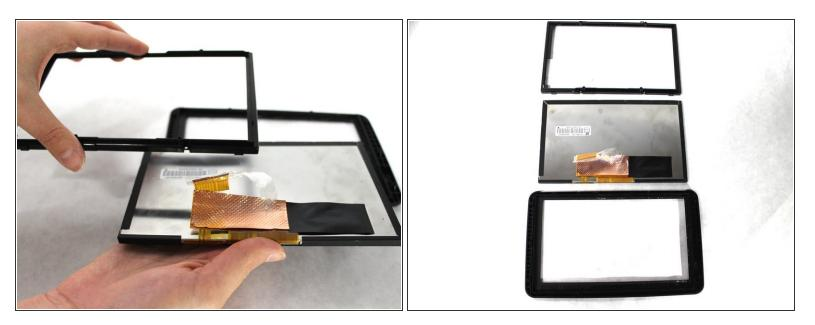
Now remove the front casing and back casing away from the screen. You will end up with three separate pieces.
