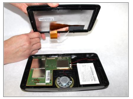
Locate the ribbon attached to the motherboard. Carefully detach the ribbon.
