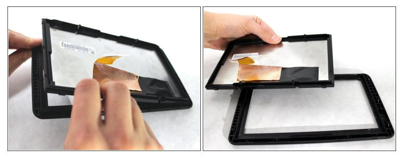
• Now pulling up on one of the corners, bring the top half of the casing out of the bottom half.
