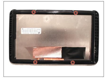
Using your T-4 Torx Screwdriver, unscrew the four 2.38 mm Torx T-4 screws from the back of your screen.
