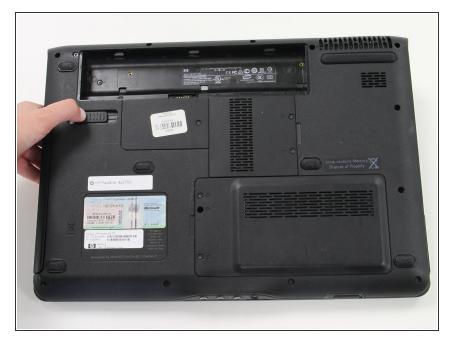
To remove the battery, pull the tab to the left and lift the battery from the computer.
