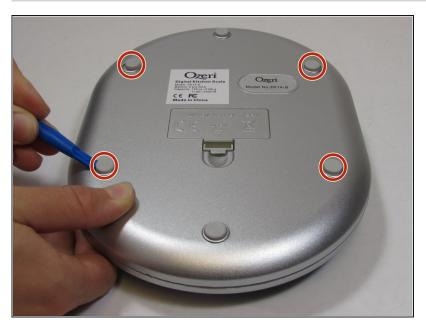
Using the iFixit opening tool, pry off the two rubber stubs on the right side and the two rubber stubs on the left side of the bottom of the device.
