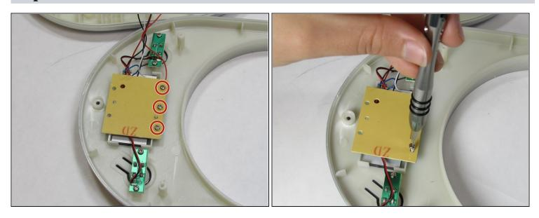
• Using the <u>2.0 Flathead</u> screwdriver, remove the three 7.20 mm screw on the back of the center LCD motherboard.
