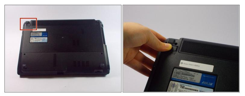
Slide the left lock button into the unlock position and hold.
