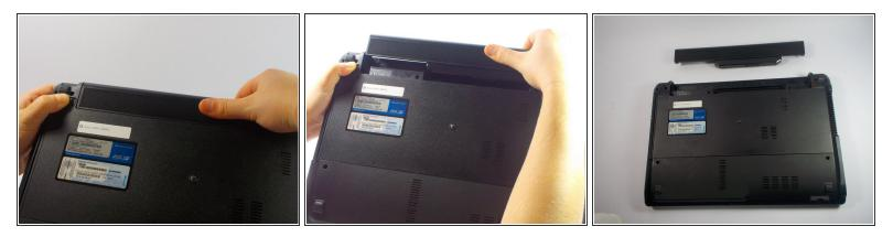
• While holding the left lock button in the unlock position, push the battery from the center away from you.
