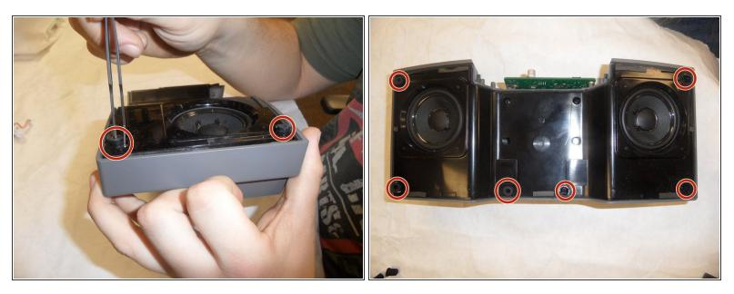
Use a wide nose tweezer to remove six rubber grommets from the front of the SoundDock XT.
