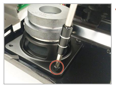
Remove the four 8.5 mm retaining screws using a # 2 phillips screwdriver.
