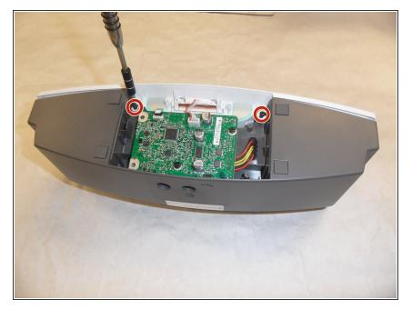
Remove the Front Panel, use a #2 Phillips screwdriver to remove the two 6.5 mm length front panel screws located under the bottom cover (highlighted in red circles in the photo).
