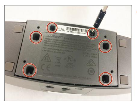
Remove six 10 mm length screws from the bottom panel of the SoundDock.XT using a #1 Phillips screwdriver.
