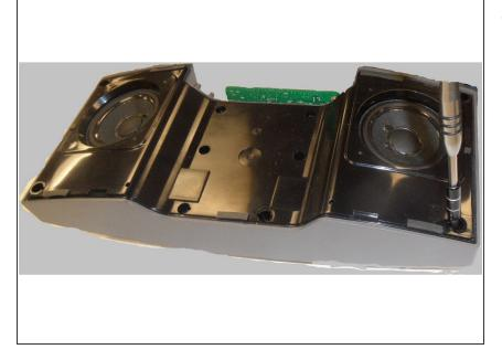
• Use a #2 screwdriver to remove the six 8.5 mm length screws from the speaker cover.
