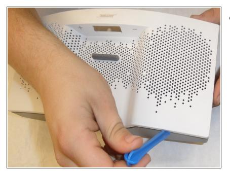
Next, use a plastic opening tool to slide under the edge of the front cover. Start edge located at the top of the left or right speaker and work your way around the speaker.
