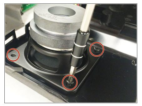
• Place and secure the new speaker using the four 8.5 mm # 2 screws.
