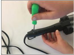
Remove all of the screws on the back of the plastic covering.
