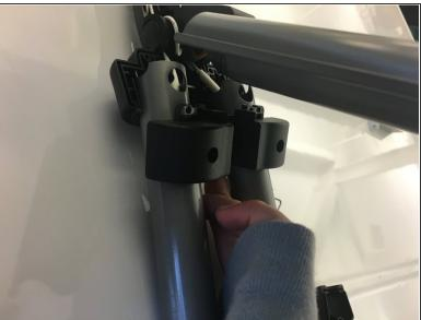
Remove the plastic cylinder holders by lifting them up and along the length of the cylinder.
