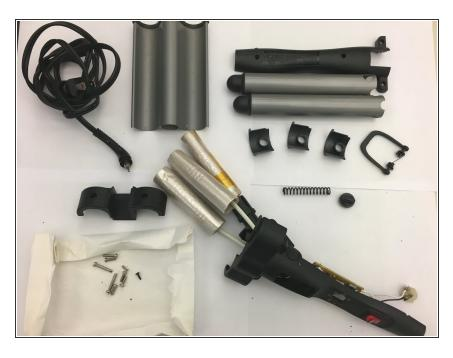
Here are all of the safely removeavable components of the waver
