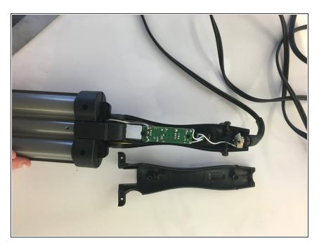
Remove the plastic handle cover by lifting it straight up.
