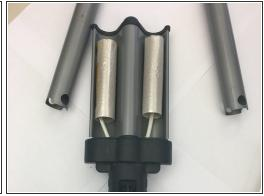
Remove the two metal cylinders by sliding them down the length of the inner soft cylinders.
