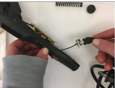
Remove the power cord from the power port of the Waver by holding the port with one hand and pulling on the cord with the other hand.
