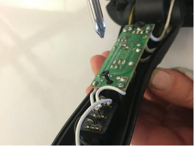
Remove the small black screw that is holding the circuit board in place.
