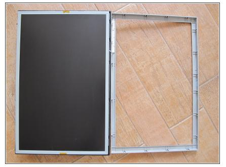
Silver edge cover unlocked. Note that a cable connects to the body.
