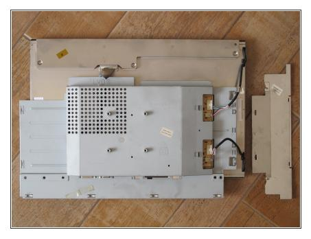
Remove the cover on the right to reveal two cables with four connectors. There is also a connector under the air holes which is now shown above the bracket with words "LVDS". Remove them all to free the metal bracket with the circuit boards from the panel.
