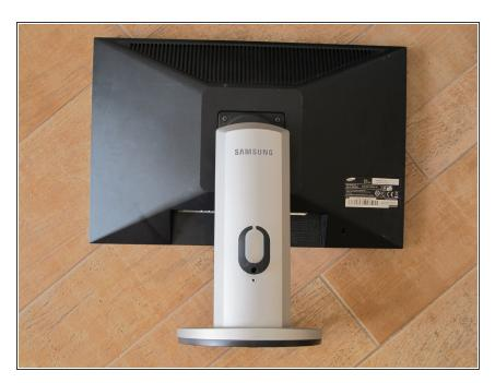
Back of the monitor. Remove the two screws at the top of the stand.
