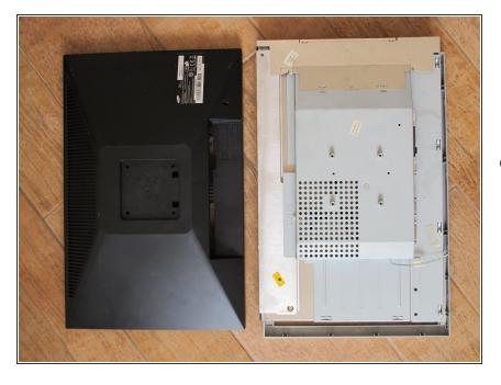
Silver edge removed and placed under the body with metal back. Black cover removed. The front panel cable connects to the bottom right of the body. Remove it. Remove the metal cover on top right by pulling it slightly on the edge at the top. This allows the two hooks on the slanting edge of the metal bracket to be unhooked.
