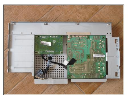
The metal bracket with circuit boards. The smaller circuit board: \* two screws (bottom left, bottom right) \* four screw extenders at the sides of the connectors The larger circuit board: \* two black screws (bottom left, top middle) \* one silver screw with washer that holds a metal strip and circuit board (top left)
