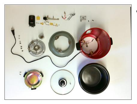
• And here we have it: a fully disassembled rice cooker.
