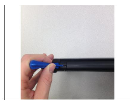
• Carefully insert your plastic opening tool into the seam and move up and down to separate the back panel from the front. Repeat this process all around the laptop until all sides have been separated.
