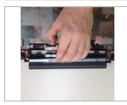
• While holding the plastic lever, gently separate the battery from the bottom panel of the laptop.
