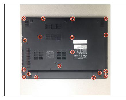
In order to access the battery you will need to remove the 18 5mm screws. Using your Phillips J1 bit remove the screws.
