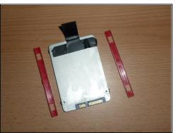
• Remove the plastic rails from the old SSD/hard drive and place them on the new SSD/hard drive.
