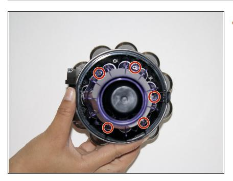
Use a T9 screw driver to remove the five 14mm screws around the edge of the cyclone body.
