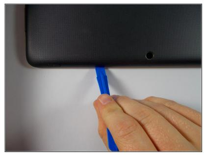
• Slide the tool along all four edges and continue to pull the tool upwards.
