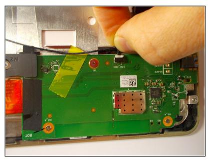
Remove the tape and unplug wire that attaches to both speakers from soundboard.
