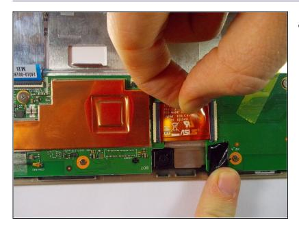
Remove black tape from ribbon cable and separate the cable from the soundboard.
