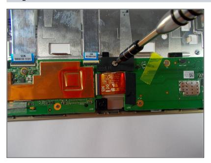
Use the +J000 screwdriver to unscrew and remove the M2 plastic holder.
