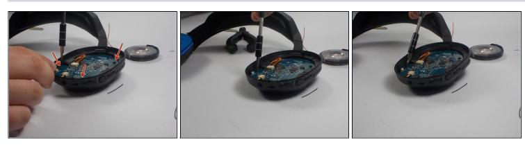
• Use screwdriver tip J00 to remove three screws fastening circuit board to casing.
