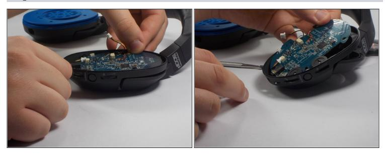
• Circuit board will be free to be removed by hand. Use plastic pry tool to slide between casing and circuit board if needed.
