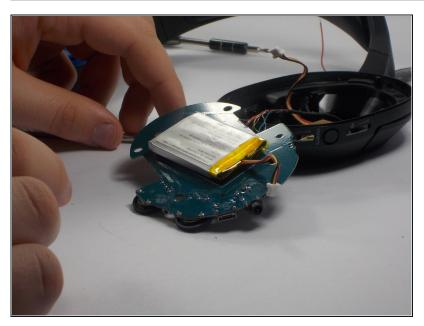
Gently removed and flip over circuit board to reveal battery pack attached to the underside. Careful not to pull out wires running through headband.
