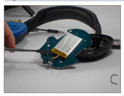
Use metal pry tool to slide between battery and circuit board to break up adhesive. Ensure the battery wire connector plug has been removed on front side.
