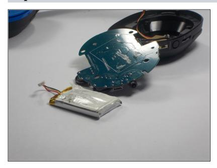
Battery will be free to be removed and replaced.
