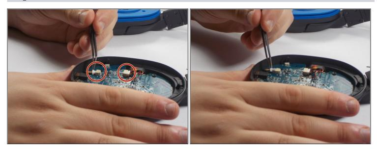
• Use bent <u>tweezers</u> to remove two wire connector plugs from circuit board.
