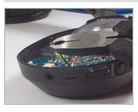
Use wire strippers to strip a portion of the rubber colored coating on the wires about a quarter inch long from both the wires connected to the circuit board and the two red and blacks wires connected to the new speaker.
