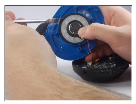
Using metal prying tool, gently slide the tool between the speaker and the blue plastic holder to break up the adhesive.
