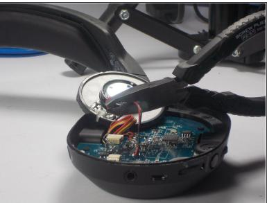
Using wire cutters, cut the red and black wires connecting the speaker to the circuit board. Be careful to leave at least one inch of wire to use reconnect wires to new speaker.
