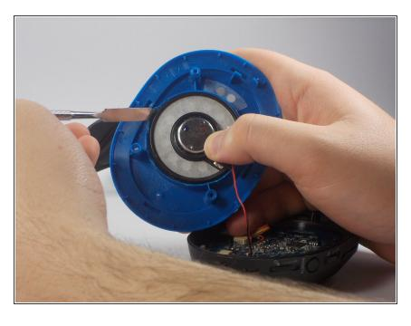
Depending on how much of the adhesive was able to be removed, you should be able to pry up the speaker assembly using plastic pry tool. If unsuccessful, use metal tool by gently working around speaker using small twisting motions until free.
