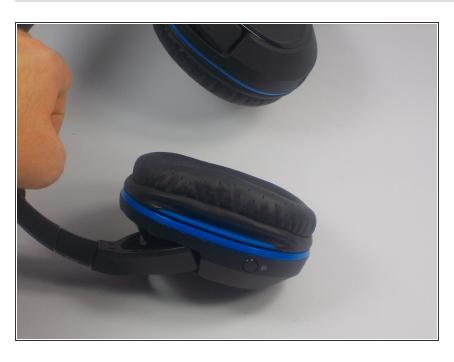
Take new ear pad, stretch, and place bottom edge over groove on edge of speaker and release.
