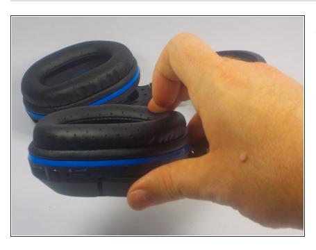
Using thumb or pointer finger from the inside of the speaker pad, push the lip of the pad into the groove on the speaker.
